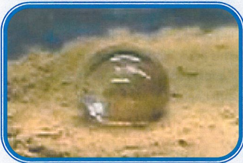
This image from Oregon State University shows a drop of water on hydrophobic (burned and waxy) soil. The droplet does not soak into the soil because of the waxy coating.
